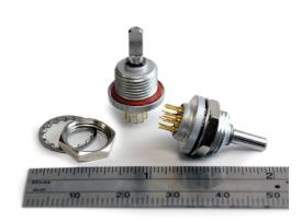
Mounting Hardware: One mounting nut .089" thick by .433" across flats and one external tooth lockwasher supplied with each switch. Mounting nut is brass, nickel plated and lockwasher is stainless steel.
